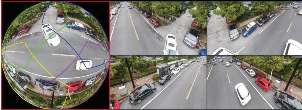
In Figure 4-83, you can adjust the color pane on the left pane or use your mouse to change the position of the small images on the right pane to realize fish eye de-warp.
